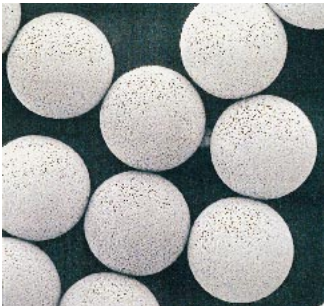
Fig. 2. Electron microscope photograph of SOURCE 15RPC. Note the uniform size distribution and the absence of broken beads and bead fragments.
